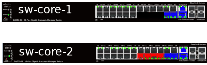
FIGURE 3 – Branchements Cisco 1 <-> Cisco 2
